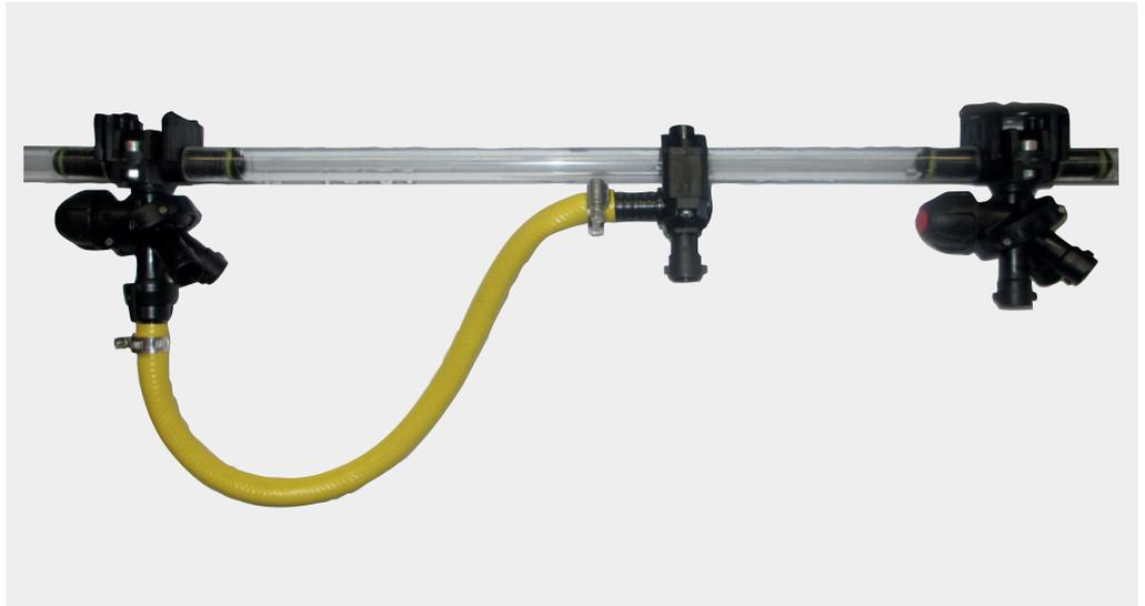
Relocation kit nozzle holder arrangement on the field spray boom
